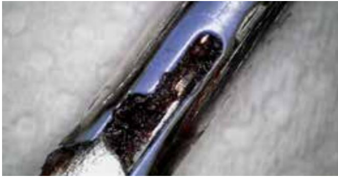
Detail of a laparoscopic forceps before BICARmed ® treatment
