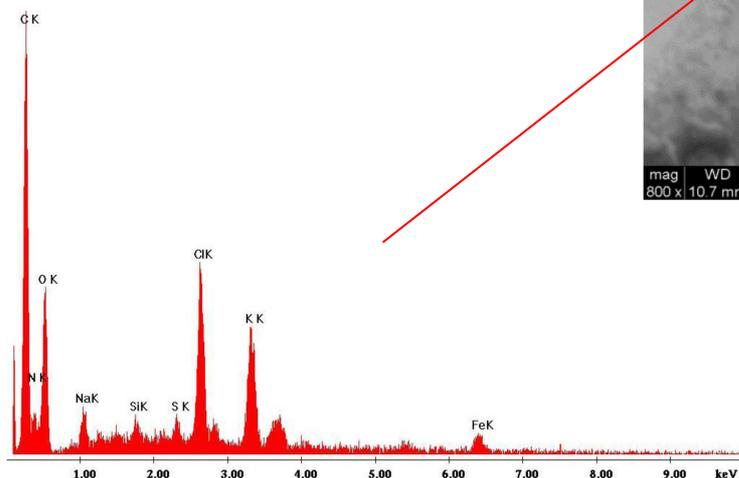
MICROANALYSIS OF PARTICLES: The main elements detected are GOLD AND IRON in the clear particle (pollutants of prepared samples, above), CARBON, CHLORINE, POTASSIUM and SODIUM in the dark particle (organic compound and saline residue)
