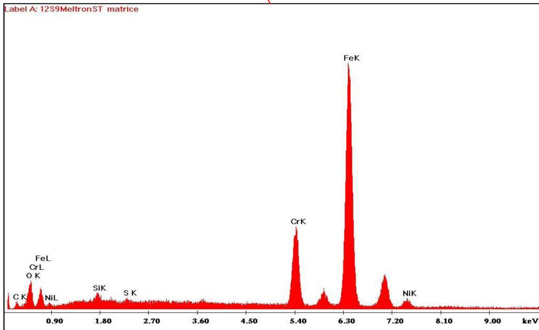
MICROANALYSIS OF THE MATRIX: The main elements detected are IRON, NICKEL, CHROME identifiable as steel
