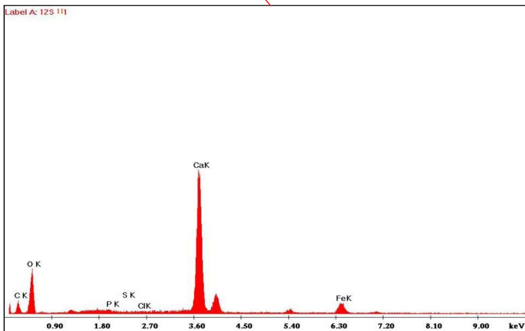
MICROANALYSIS OF SMALL PARTICLES: The main elements detected are CALCIUM, OXYGEN and IRON attributable to the saline compound containing calcium but not belonging to connective tissue residue.
