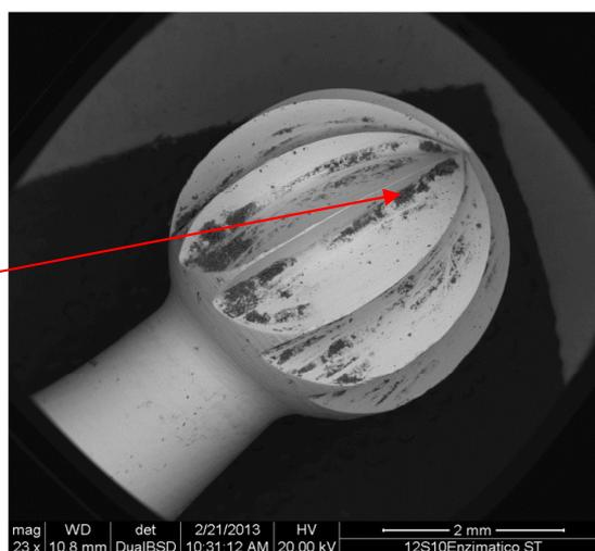
**MICROANALYSIS OF THE DARK PARTICLE:** The main elements detected are CALCIUM, PHOSPHORUS, OXYGEN (connective tissue residue)
