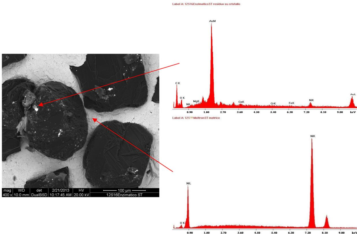
MICROANALYSIS OF THE MATRIX: The main element detected IS NICKEL (higher spectrum)
