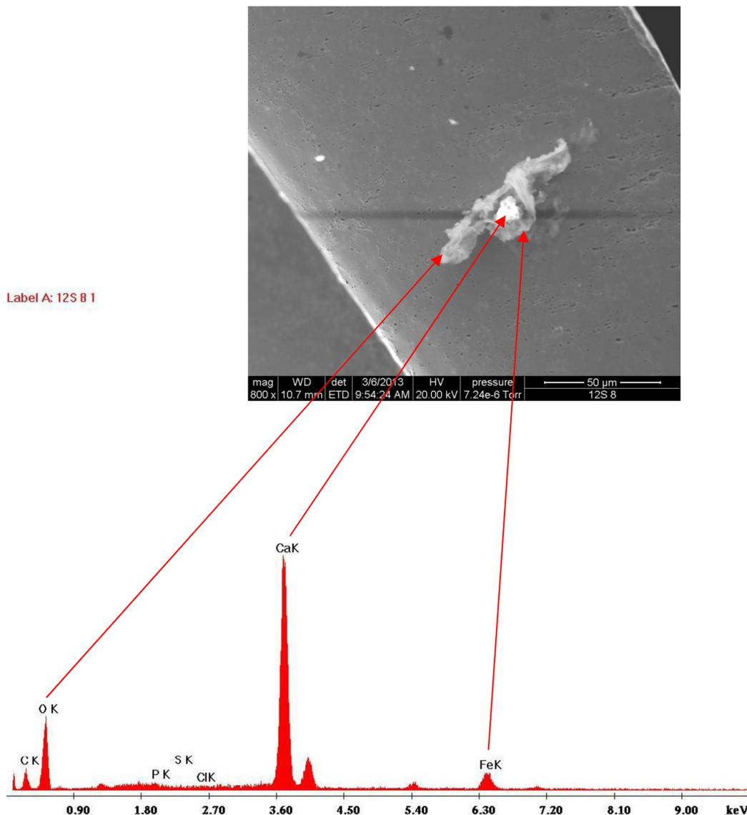
MICROANALYSIS OF THE PARTICLE: The main elements detected are CALCIUM, OXYGEN and IRON representative of the saline compound containing calcium but no connective tissue residue.
