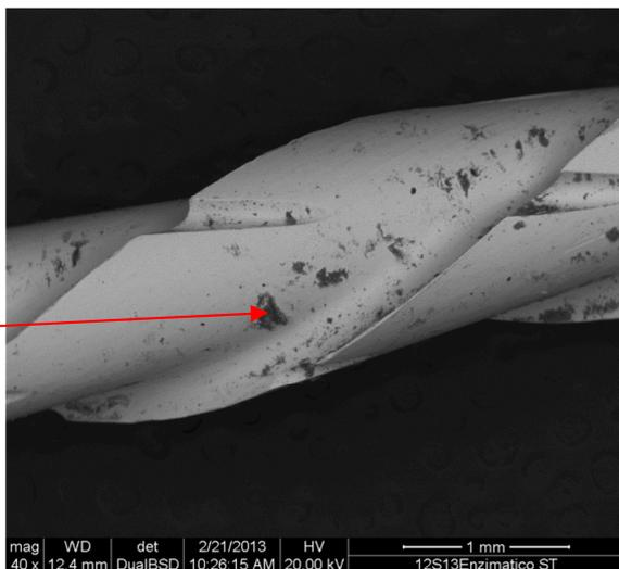
**MICROANALYSIS OF SMALL DARK PARTICLES:** The main elements detected are CALCIUM, PHOSPORUS, and OXYGEN (connective tissue residue).
