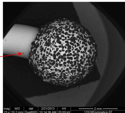
MICROANALYSIS OF PARTICLES ON STEM: The main elements detected are IRON, CHROME, and NICKEL (STEEL)
