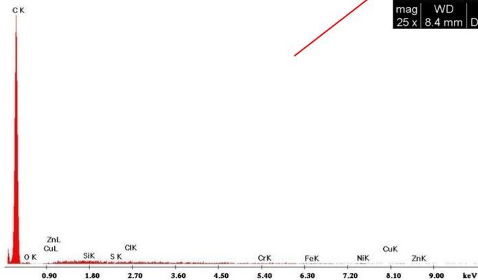
MICROANALYSIS OF PARTICLES: The main elements detected are NICKEL (higher spectrum) and CARBON (lower spectrum).
