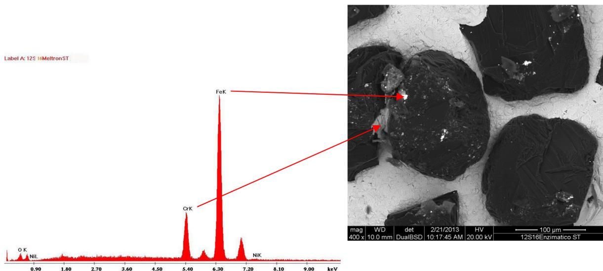
MICROANALYSIS OF THE STUCK: The main elements detected are IRON, CHROME, NICKEL (STEEL)
