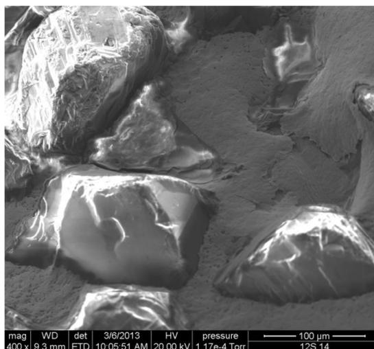
MICROANALYSIS OF GREY PARTICLES: The main elements detected are CALCIUM, PHOSFORUS, OXYGEN (comprising connective tissue residue), POTASSIUM, CHLORINE, CARBON AND SODIUM.
