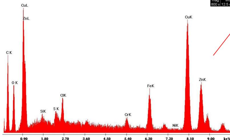
MICROANALYSIS OF THE DARK PARTICLE (higher spectrum): The main elements detected are CHLORINE, CARBON, OXYGEN comprising the saline compound.
