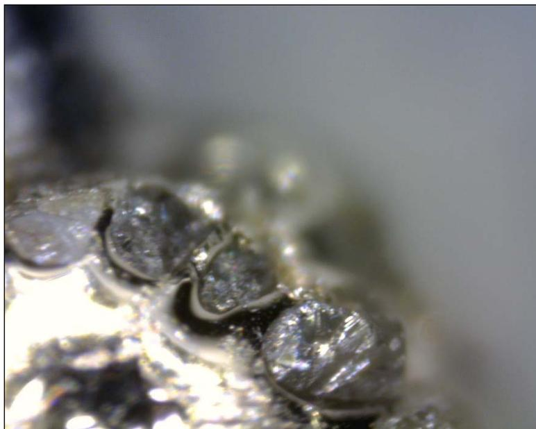
Following are pictures taken with a digital microscope of a finned milling cutter, model E8250LSO of 5 mm used in Otosurgery (ID O24) before and after the mechanical cleaning (40 seconds), done 3 days after its use.
