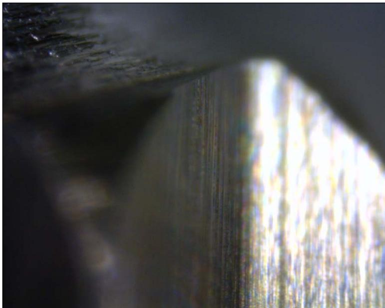
The following pictures taken with a digital microscope refer to a diamond-coated bit, model E5220 of 2 mm, used in Otosurgery (ID O22) before and after the mechanical cleaning (27 seconds), carried out 15 days after its use.
