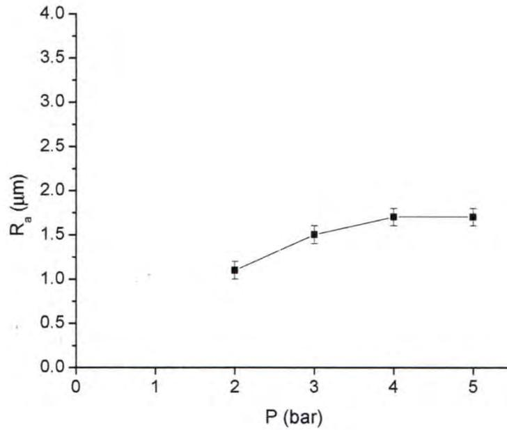
**Figure 1** Ra with various treatment pressure of a painted sample. The powder size was 0.130. The blue point refers to the untreated aluminium. The points shown refer to areas named 2a, 3a, 4a, 5a.
