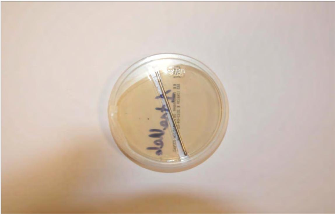
*The Petri dish containing with the drill bit decontaminated with the MELTRON® compound: No growth*
