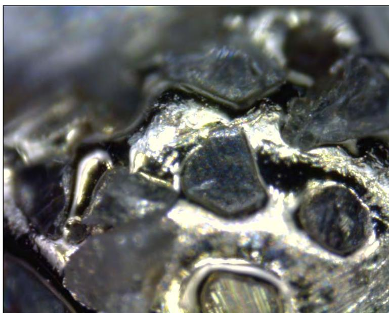
Shown below are the detailed photos taken with a digital microscope of a diamond-coated bit, model E6215 of 1.5 mm, used in Otosurgery (ID O14) before and after the mechanical cleaning (25 seconds), done 7 days after its use.
