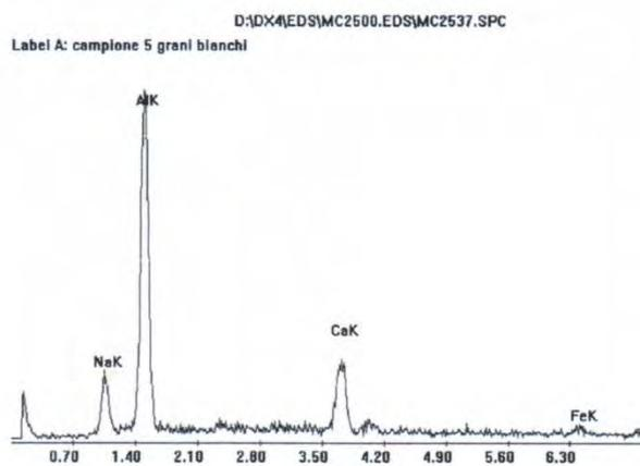
Figure 3 EDX spectra of a grain visible in Figure 2. The peaks of Sodium and calcium are clear. The peak of aluminum is mainly due to the material surrounding an under the grain.
