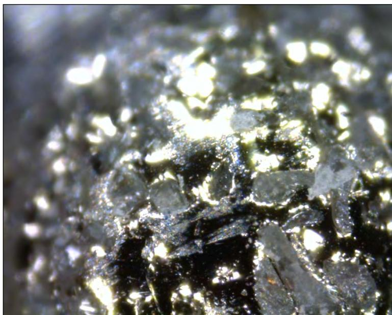
In detail, the photos to digital microscope of a milling cutter finned model E8040LSO 4 mm used in Otosurgery (ID OL5) before and after the mechanical cleaning (27 seconds with MELTRON® GG, at 10 cm from the nozzle MINIJET®), operated after a few hours of use.
