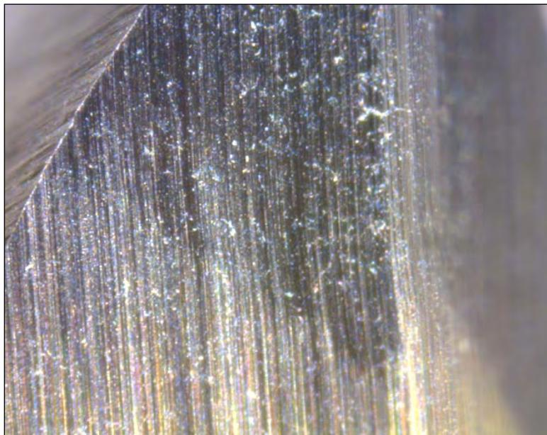
The table shows the photos to digital microscope of a craniotome model GE520R used in Neurosurgery (ID N6) before and after the mechanical cleaning (48 seconds with MELTRON® GG, at 10 cm from the nozzle MINIJET®), on the same day use.
