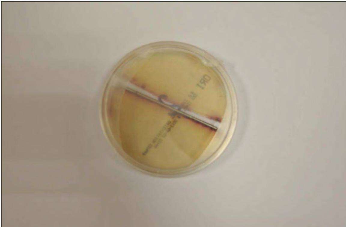
*The Petri dish containing with the untreated drill bit: 20 colonies of E. Coli*
