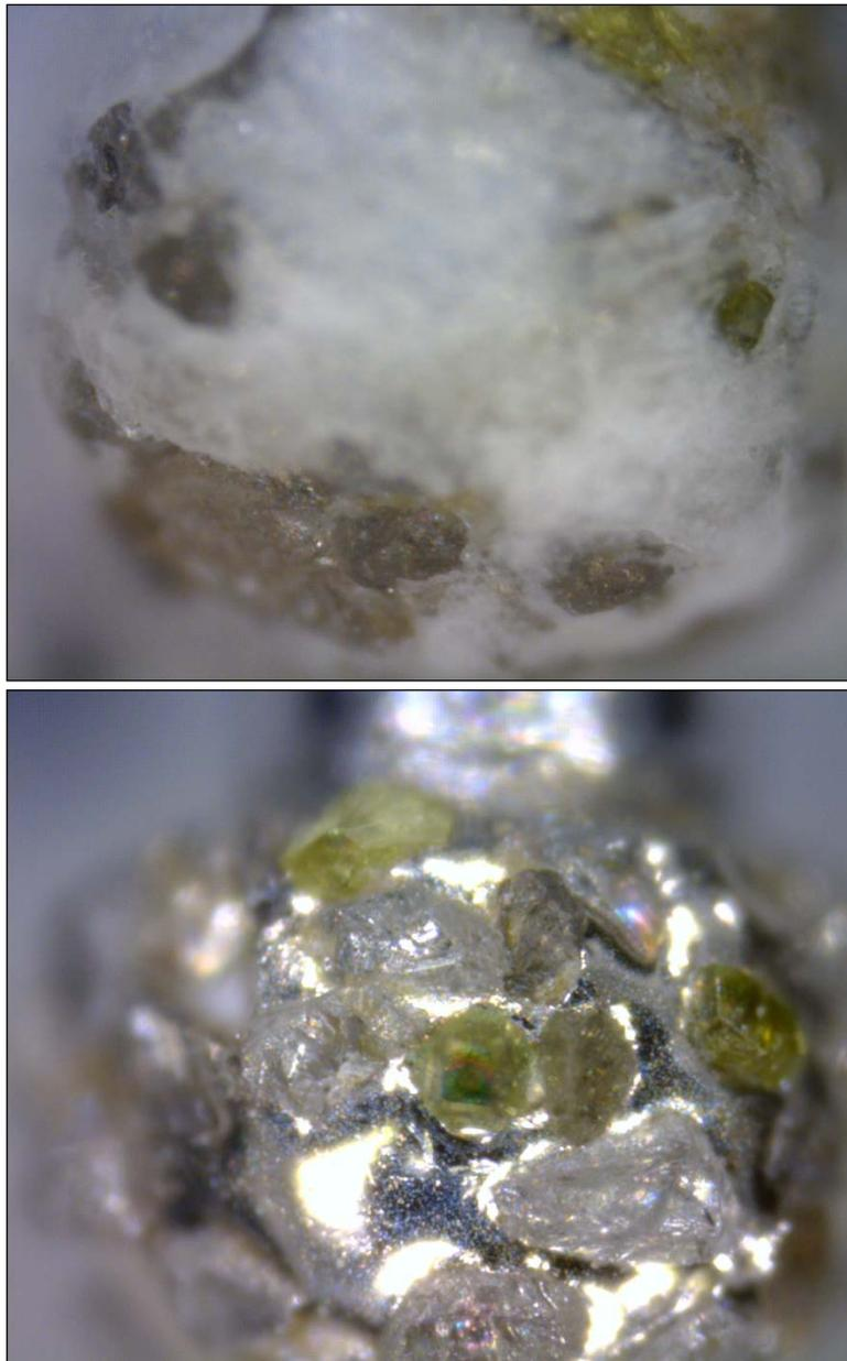
Following are the photos taken with a digital microscope of a diamond-coated bit model E6207 of 0.7 mm used in Otosurgery (ID O15) before and after the mechanical cleaning (33 seconds with MELTRON® FX, to 2/3 cm from the nozzle and a pressure MICROJET® out of 4 bar), implemented 2 days after its use.
