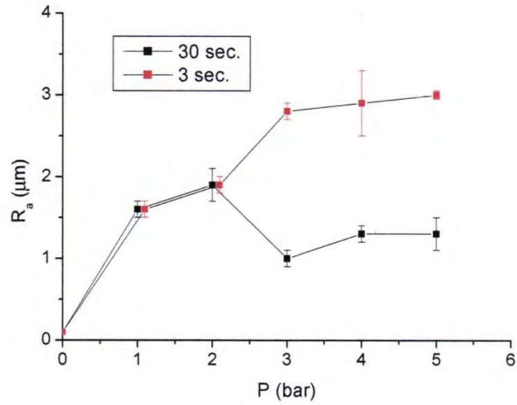
**Figure 3** Ra with various treatment pressure of 2024 T3 Alclad alloy. The powder size was 0.130.
