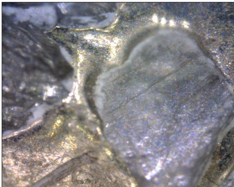
Following are pictures taken with a digital microscope of the shank of a diamond-coated bit model E5050 of 5 mm used in Otosurgery (ID O7) before and after the mechanical cleaning implemented 1 day after its use in the ward. (35 seconds, with MELTRON® GG, at 10 cm distance from the nozzle MINIJET® with rinsing at the end).
