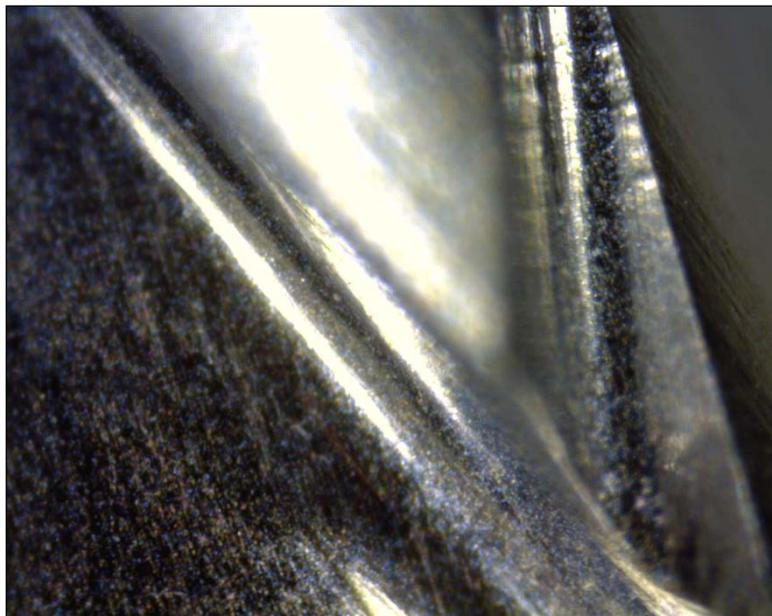
The two pictures below taken with a digital microscope refer to a diamond-coated bit, model E5130 of 6 mm, used in Otosurgery (ID O18) before and after the mechanical cleaning (30 seconds), which took place 1 day after its use.
