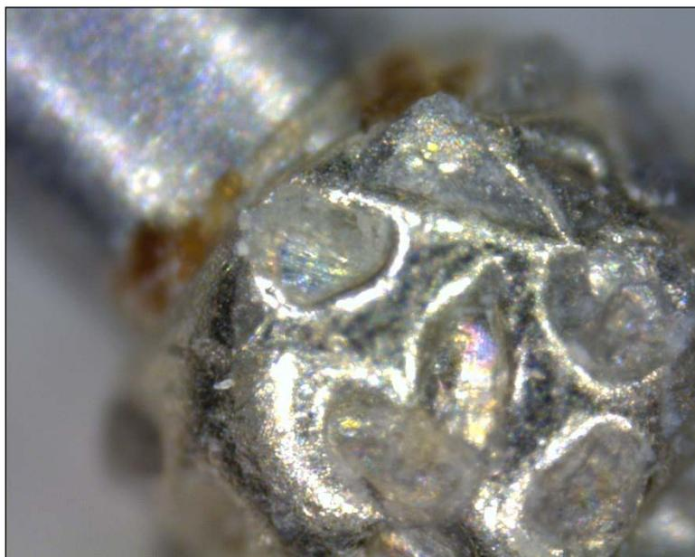
Shown below are the detailed pictures taken with a digital microscope of a finned bit model GE504R 2.3 mm used in neurosurgery (ID N2) before and after the mechanical cleaning (30 seconds), performed after one day of use in the ward.
