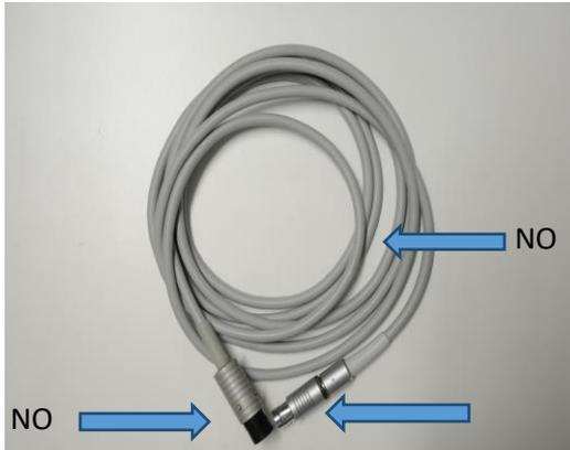
Only the steel ends can be treated, not the plastic hose.
