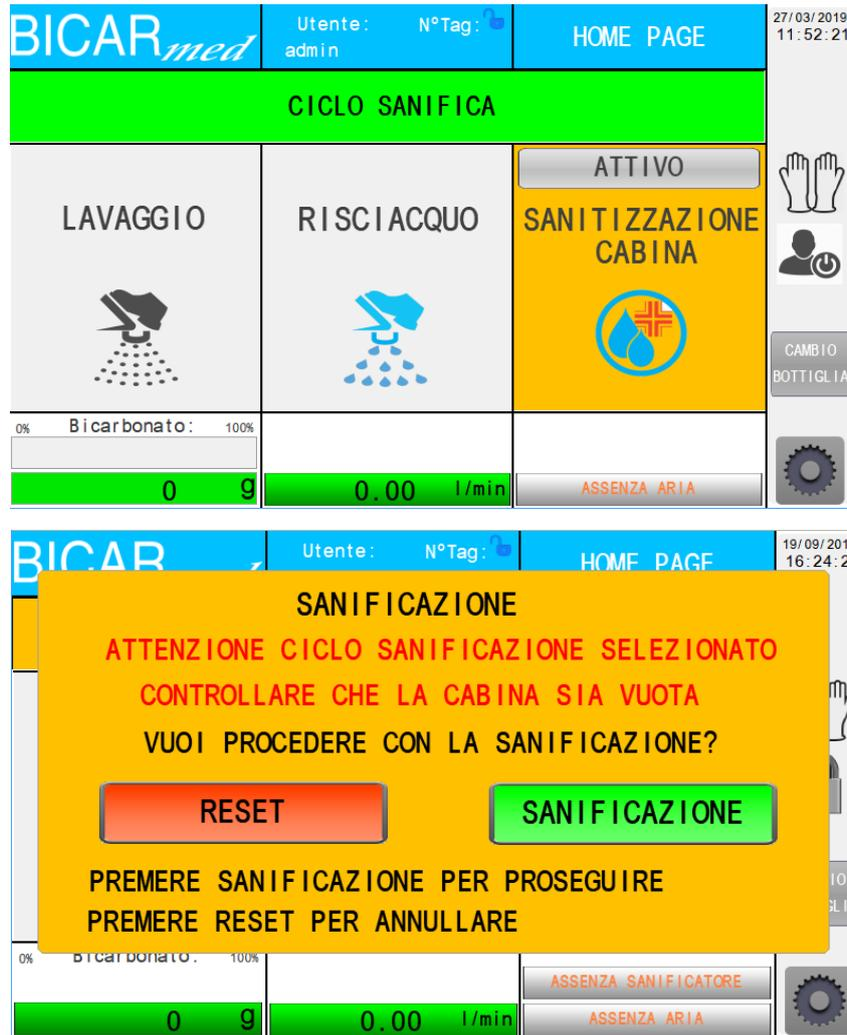
Sanitization cycle selected; press the sanificazione (sanitization) button to start or press the reset button to cancel.
