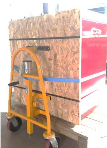
The machine can therefore be moved using suitable lifting equipment or by placing two trolleys / sliding blocks under the bench, at the junctions between the central and side sections.
