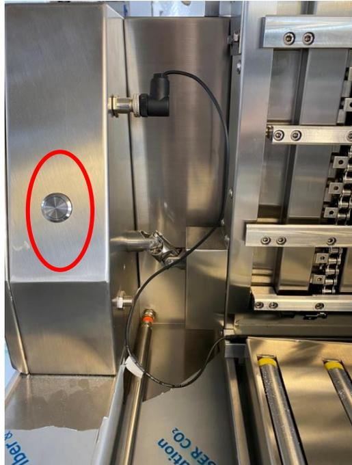
Once the tray loading procedure has been completed, you can make a tray call from inside the cabin by pressing the "tray call" button on the push button panel.
