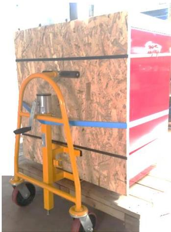
After opening the box, the machine must be lifted with special equipment designed for moving furniture.
