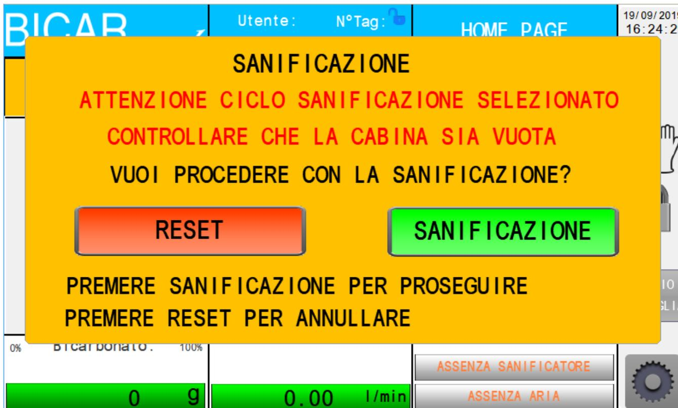
Press the SANITIZATION softkey or cancel the cycle by pressing the RESET softkey.
