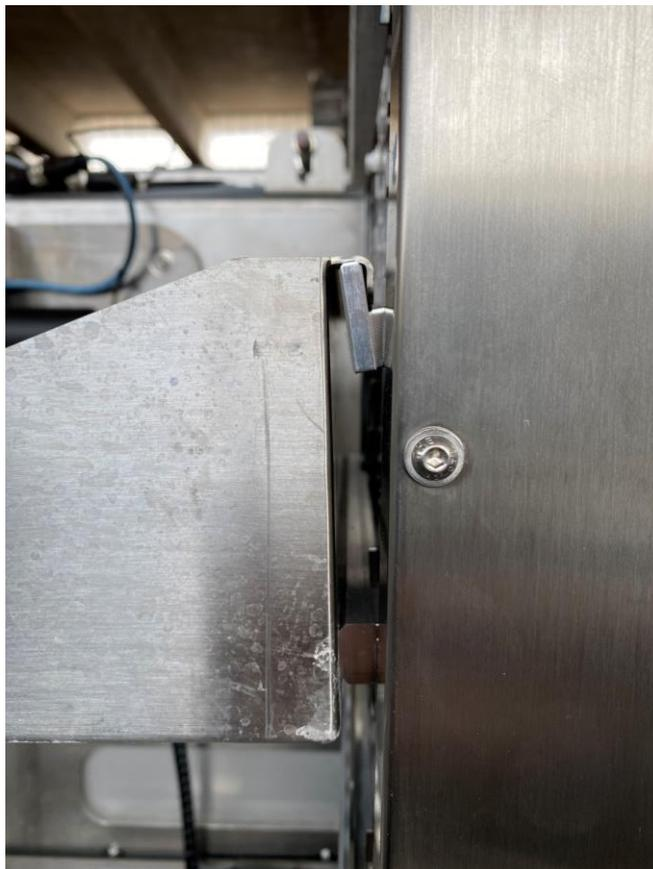
To free up the lowest position in the loader automatically, you can load a tray and then press the button on the box at the side of the tower. This function will move the previously loaded tray up by one position. The tower has 5 positions in which trays can be loaded. The maximum load sensor is located at the top on the side of the cabin. Once engaged, it will not allow the tower to move upwards.
