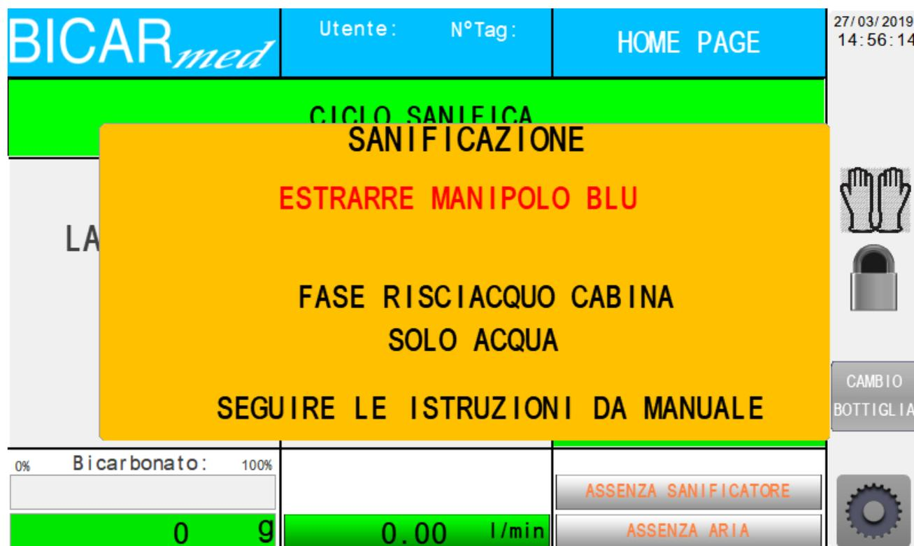
During this phase, only water will automatically come out of the blue handpiece to rinse the surfaces inside the cabin.
