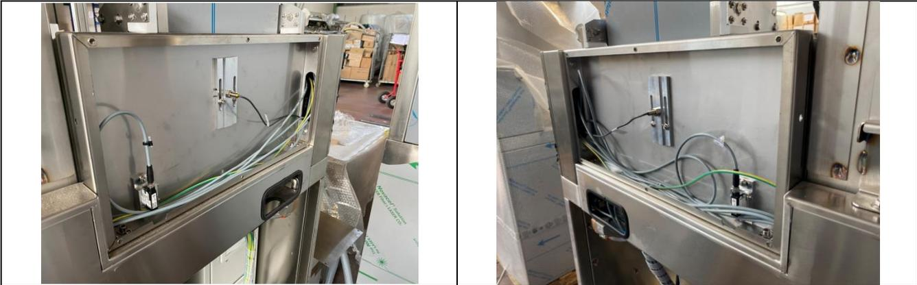
Open the side of the motor boxes and make the electrical connections following the wiring diagram.
