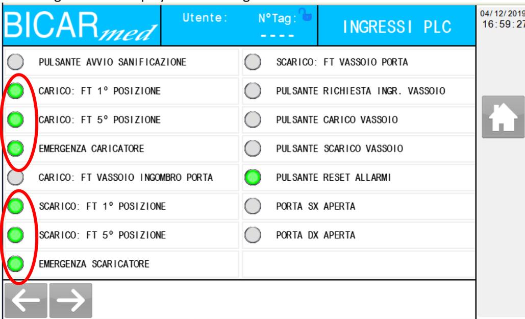
Check that there is a green light on the sensors circled in red. Check under LOAD: TRAY OVERALL DOOR PHOTOCELL and UNLOAD: TRAY DOOR PHOTOCELL that the light is grey.
