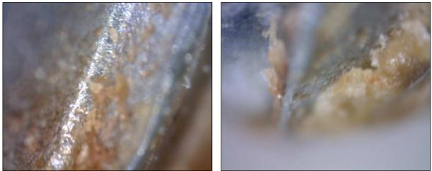
Cleaning: 60 seconds exposure to MELTRON<sup>®</sup> GG Pressure 3.5 bar - Distance 5 - 10 cm – Rinsing and Blowing
