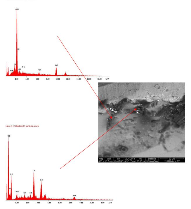
MICROANALYSIS OF PARTICLES: The main elements detected are GOLD AND IRON in the clear particle (pollutants of prepared samples, above), CARBON, CHLORINE, POTASSIUM and SODIUM in the dark particle (organic compound and saline residue)
