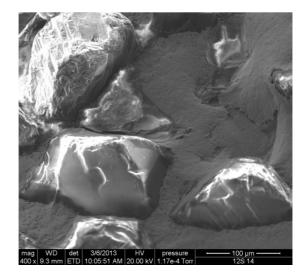
MICROANALYSIS OF GREY PARTICLES: The main elements detected are CALCIUM, PHOSPORUS, OXYGEN (comprising connective tissue residue), POTASSIUM, CHLORINE, CARBON AND SODIUM.
