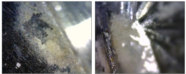
Cleaning: 60 seconds exposure to MELTRON<sup>®</sup> GG Pressure 3.5 bar - Distance 5 - 10 cm – Rinsing and Blowing
