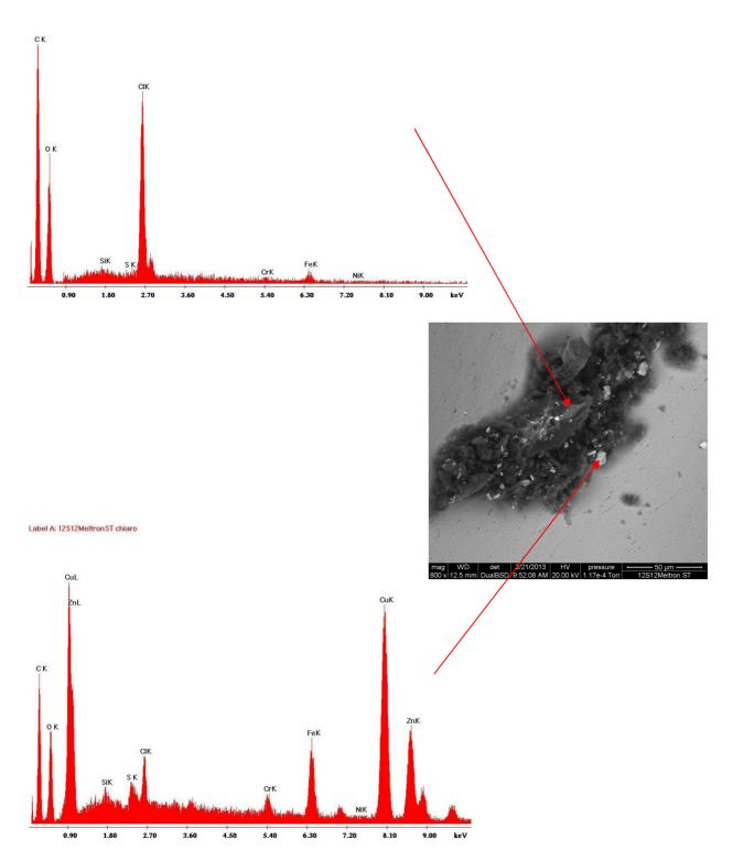
MICROANALYSIS OF THE DARK PARTICLE (higher spectrum): The main elements detected are CHLORINE, CARBON, OXYGEN comprising the saline compound.
