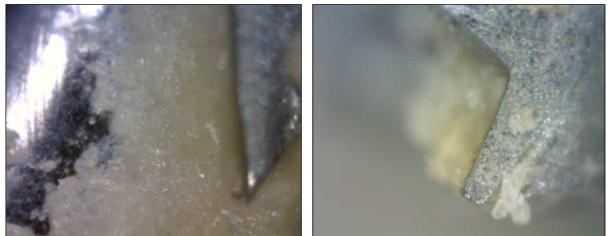
Cleaning: 45 seconds exposure to MELTRON<sup>®</sup> GG Pressure 3.5 bar - Distance 5 - 10 cm – Rinsing and Blowing
