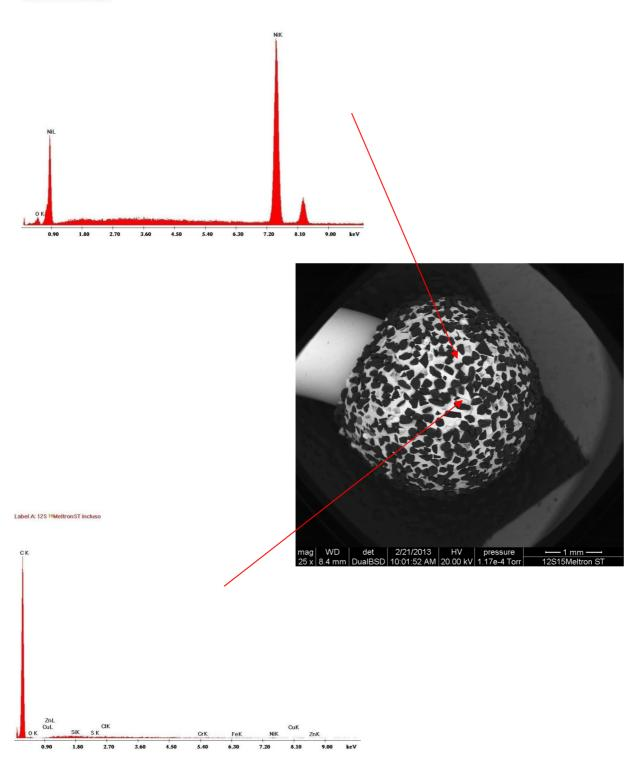
MICROANALYSIS OF PARTICLES: The main elements detected are NICKEL (higher spectrum) and CARBON (lower spectrum).
