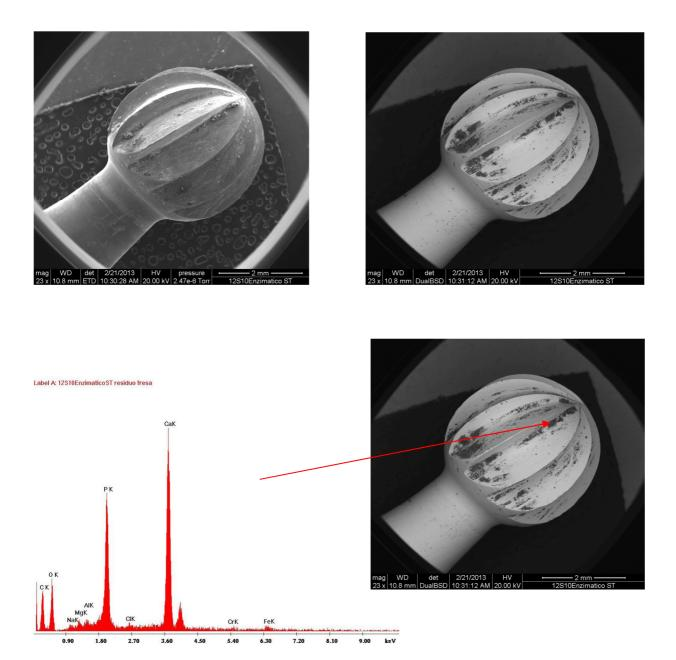
MICROANALYSIS OF THE DARK PARTICLE: The main elements detected are CALCIUM, PHOSPHORUS, OXYGEN (connective tissue residue)
