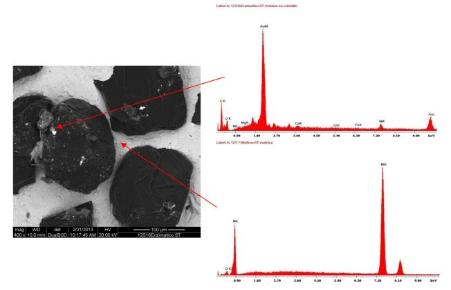
MICROANALYSIS OF THE MATRIX: The main element detected IS NICKEL (higher spectrum)
