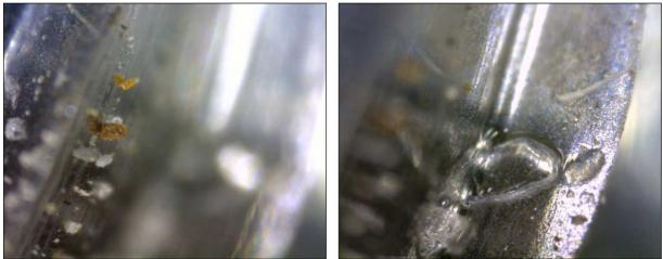
Cleaning: 30 seconds exposure to MELTRON<sup>®</sup> GG Pressure 3 bar - Distance 5 - 10 cm – Rinsing and Blowing
