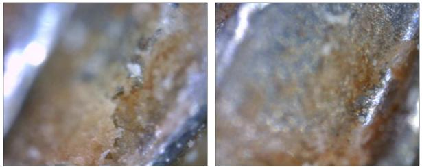
Cleaning: 50 seconds exposure to MELTRON<sup>®</sup> GG Pressure 3.5 bar - Distance 5 - 10 cm – Rinsing and Blowing
