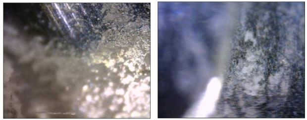
Cleaning: 60 seconds exposure to MELTRON® GG Pressure 3.5 bar - Distance 5 - 10 cm – Rinsing and Blowing
