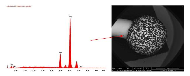
MICROANALYSIS OF PARTICLES ON STEM: The main elements detected are IRON, CHROME, and NICKEL (STEEL)
