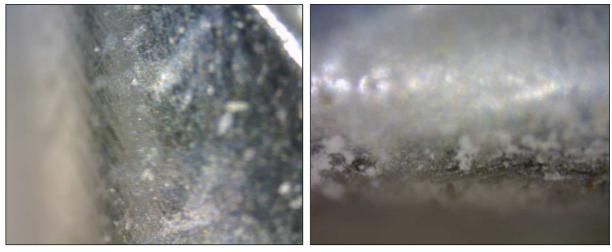
Cleaning: 30 seconds exposure to MELTRON<sup>®</sup> GG Pressure 3.5 bar - Distance 5 - 10 cm – Rinsing and Blowing
