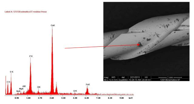
MICROANALYSIS OF SMALL DARK PARTICLES: The main elements detected are CALCIUM, PHOSPORUS, and OXYGEN (connective tissue residue).
