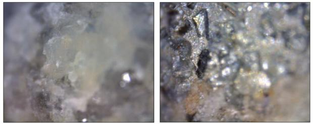
Cleaning: 80 seconds exposure to MELTRON<sup>®</sup> GG Pressure 3.5 bar - Distance 5 - 10 cm – Rinsing and Blowing
