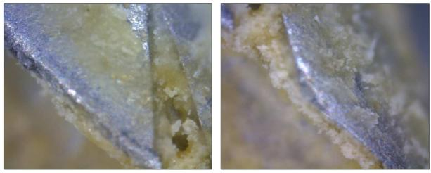
Cleaning: 40 seconds exposure to MELTRON® GG Pressure 3.5 bar - Distance 5 - 10 cm – Rinsing and Blowing
