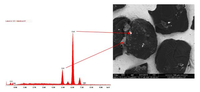
MICROANALYSIS OF THE STUCK: The main elements detected are IRON, CHROME, NICKEL (STEEL)
