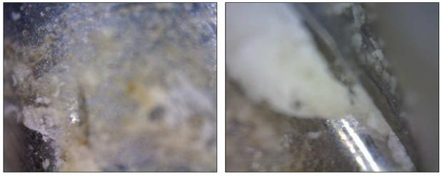
Cleaning: 30 seconds exposure to MELTRON<sup>®</sup> GG Pressure 3 bar - Distance 5 - 10 cm – Rinsing and Blowing
