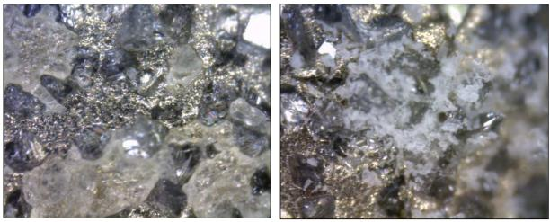
Cleaning: 30 seconds exposure to MELTRON® GG Pressure 3.5 bar - Distance 5 - 10 cm – Rinsing and Blowing
