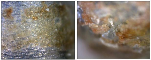
Cleaning: 43 seconds exposure to MELTRON<sup>®</sup> GG Pressure 3.5 bar - Distance 5 - 10 cm – Rinsing and Blowing
