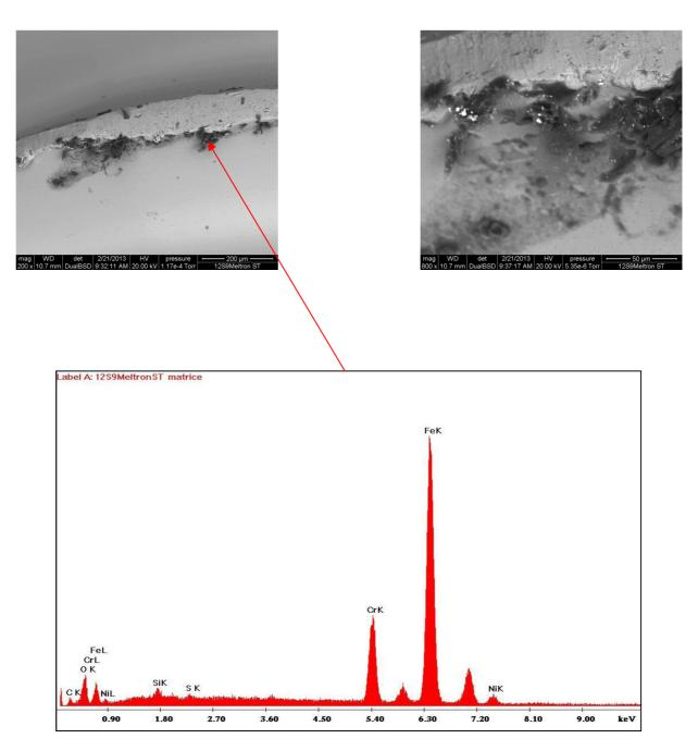
MICROANALYSIS OF THE MATRIX: The main elements detected are IRON, NICKEL, CHROME identifiable as steel
