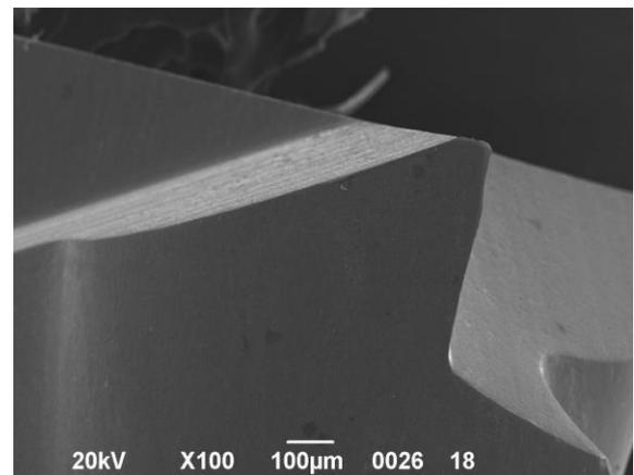
The samples of group 1 showed surfaces particularly altered after the standard cleaning treatment. In the craniotome case on the surface it were identified some particles whose total area represented 4.19% of the total area of the craniotome itself; these particles have a uniform chemical composition: calcium, phosphorus, oxygen (bone tissue residue) and other trace elements, these data were obtained by scanning electron microscope (SEM) analysis.
