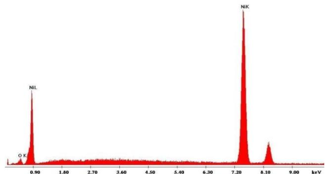
MATRIX MICROANALYSIS: main element found is NICKEL (upper spectrum)
