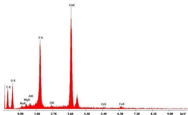
DARK PARTICLE MICROANALYSIS: main elements found are CALCIUM, PHOSPHORUS, OXYGEN (bone tissue residue)
